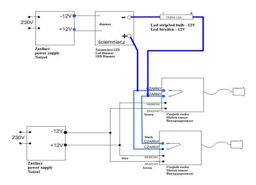
On / off system using LED strip / LED bulbs 12V with an additional button attached enabling all the lighting points to be
