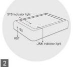
Smart Link Mode Press 'RST'( The SYS indicator light flickers, the LINK indicator light flashes.)
