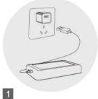
Power Connection Supply power for the device with USB power adapter, DC5V/500mA.
