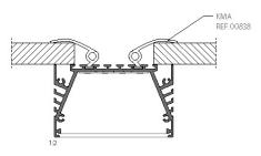
\* Zalecamy użycie dwóch spręzyn GP na maksymalnie 50 cm profilu / \* We recommend the use of two GP springs for lamps with a max. Length of 50 cm. / \* We recommend the use of two GP springs for lamps with a max. Length of 50 cm.
