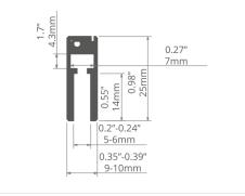
Easy and secure mounting to panel edges. Convenient installation of led strips. Adapted for panels with a thickness of (0.23" / 5-6 mm).
