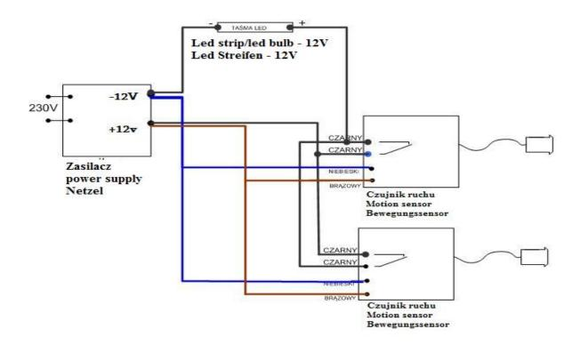
On / off system using led strip / led bulbs - 12V and with an attached dimmer for adjusting the light intensity
