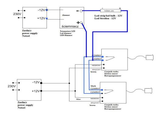
On / off system using LED strip / LED bulbs 12V with an additional button attached enabling all the lighting points to be
