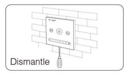
Plug into the below bayonet with a screwdriver, and upwarp screwdriver, then you can dismantle the controller.
