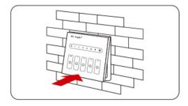
Clicks into the upper side of panel dimmer base, then press the lower side slightly to make it clicks into the base.
