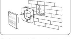
Fix the panel dimmer base on the bottom case with screw.
