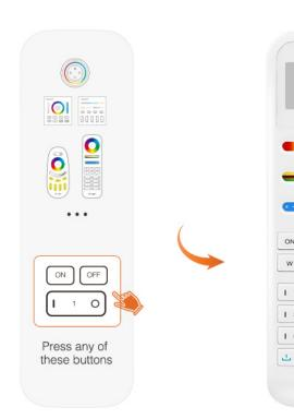
2. Within 10 seconds Short press any buttons of 2.4GHz series remote once
