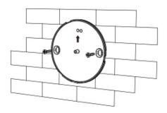
2. Install battery(AAA battery•2pcs), then fix it on the base.
