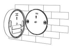
3. Press downward and rotate to the left to fix it.
