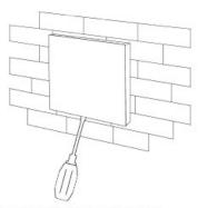
Plug into the below bayonet with a screwdriver, and upwarp screwdriver, then you can dismantle the controller.
