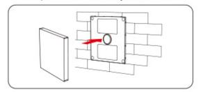
4. Put the rotating switch on the front of holder
